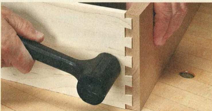
▲ You want to shoot for an easy-to-assemble fit between the pins and the tails. It shouldn't take more than a few light taps with a mallet to seat the tails flush with the pins.
