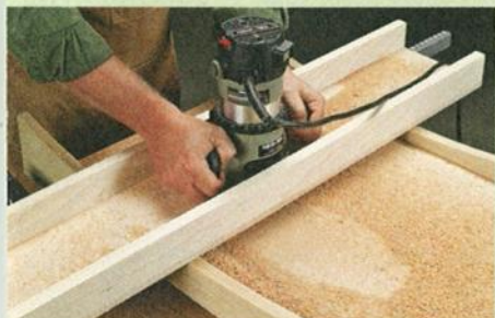
Shop-Made Router Jig. You'll find details on the jig I used to shape the seat on page 28.
